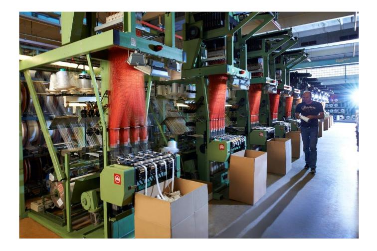
In Altshausen our ribbons are manufactured on different ribbon weaving machines and crocheting machines of the leading manufacturers Comez, Jakob Müller and Mageba.
